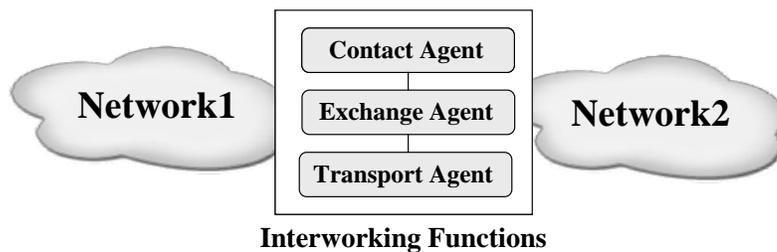
**Figure 11: Agent-based Architecture of IWF**
