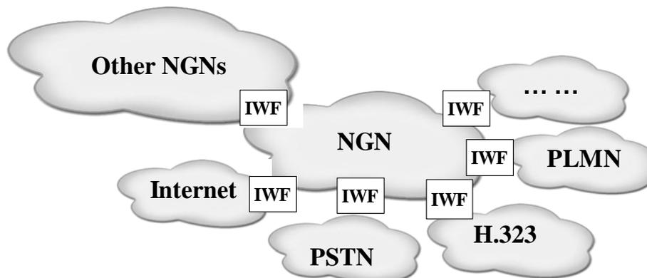
**Figure 9: Requirements for Interworking with legacy networks**
