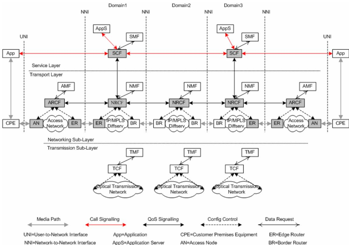
**Figure 8: Reference model of End-to-end QoS architecture (Source: ITU-T)**
