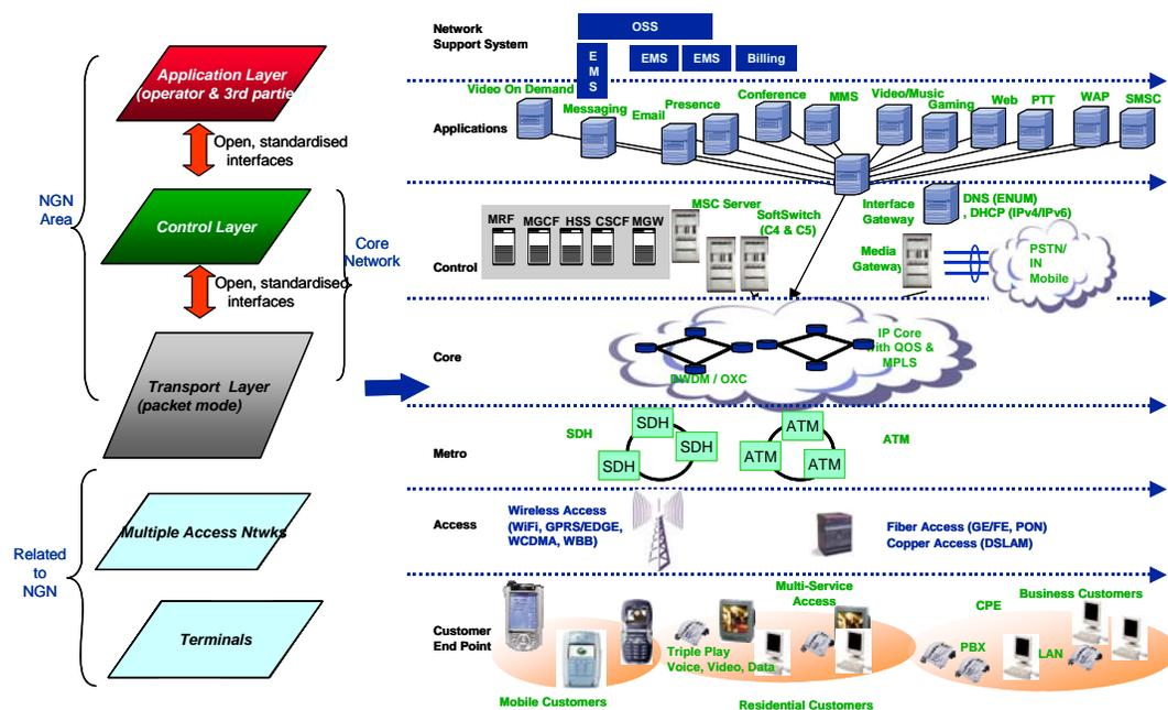
Figure 2: NGN Layered Architecture Model (Source: ITU-T)
