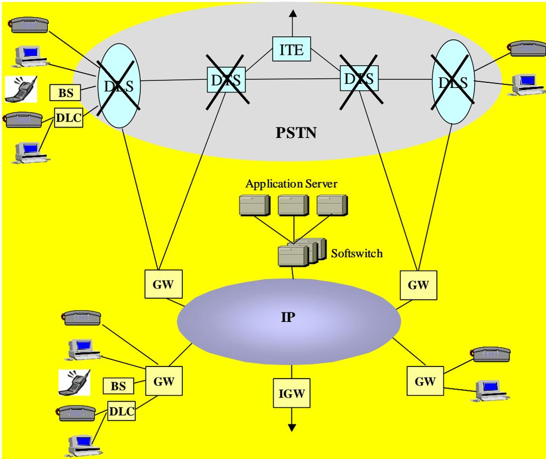
Figure 4: Phasing out of TDM switches and full NGN implementation roll out
