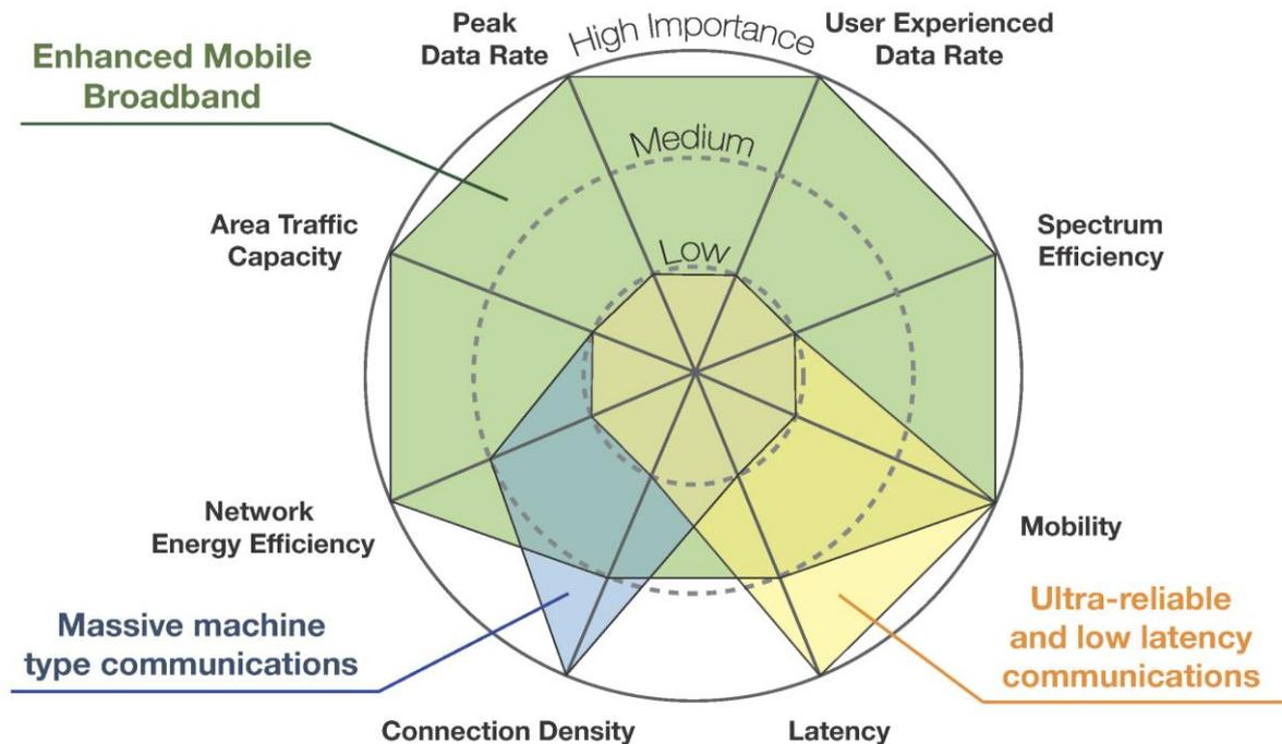
**Figure 5 – The importance of key capabilities in different usage scenarios**
